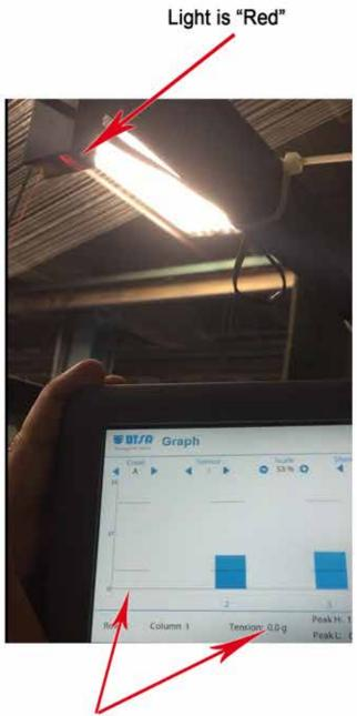
When Yarn is removed, tension drops to 0g, light turns Red, and alert/stop signal is activated.
